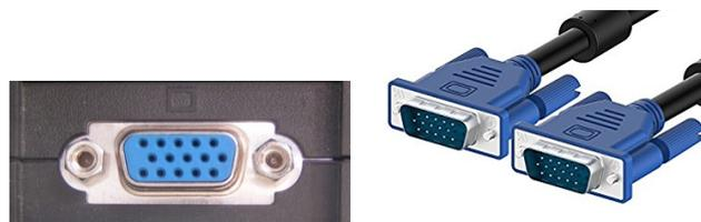
If you do not have a standard HDMI port or VGA port on your computer, you will need a display adapter to connect the standard HDMI cable or VGA cable to your computer's display port (e.g., "HDMI to Mini DisplayPort (Mac)", "HDMI to Mini HDMI", "HDMI to Micro HDMI", "VGA to Mini DisplayPort (Mac)").
